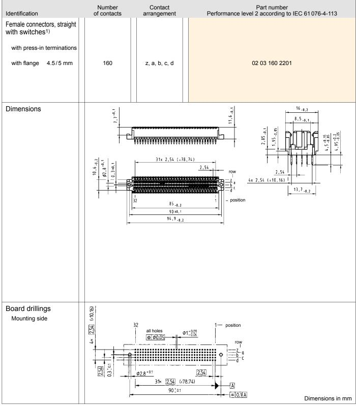
$^{1)}$  Switching elements at positions a21-22, b4-5, b6-7, b8-9 and b10-11 Further types see DIN 41612 catalogue
