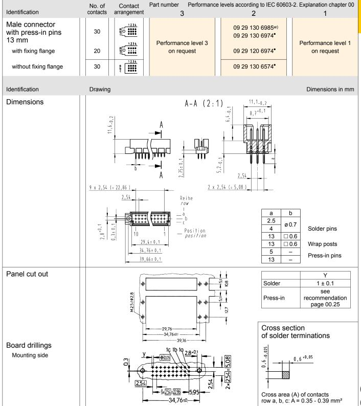
Other contact arrangements as well with lagging/leading pins on request • Wrap posts for interfacing selectively gold plated (performance level 3)
