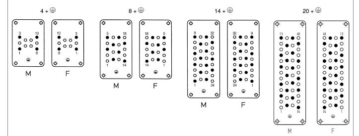
$\bullet \ \text{Working contact} \quad \circ \ \text{Without contact} \quad \text{M - Male insert} \quad \text{F - Female insert}$
