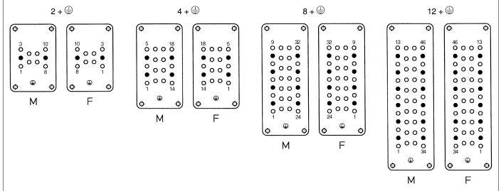
• Working contact O Without contact M - Male insert F - Female insert
