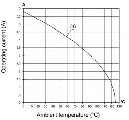
0  $\,$  6 B hoods/housings with 2 modules Conductor cross-section 0.5  $mm^2$
