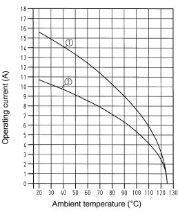
① 24 B hoods/housings with 6 modules Conductor cross-section 2.5 mm<sup>2</sup>
