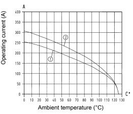
0 24 B hoods/housings with 3 modules Conductor cross-section 50  $\textrm{mm}^2$
